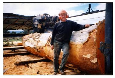
All the stringy bark logs had to be barked because the fibres of the bark would get caught in the bearings of the break down saw and it would run hot. Barking wasn't too bad of a job in the spring and through the summer, but when the winter come, the bark could seize up because they weren't growing. So that made it a hard job.
